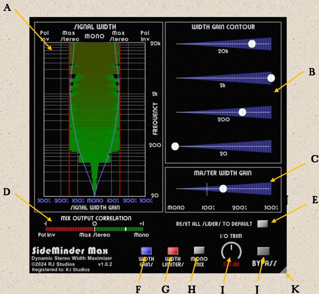
**A – Activity Display** – provides multiple pieces of information over the audio spectrum from 20 Hz at the very bottom of the display to 20kHz at the top of the display:
